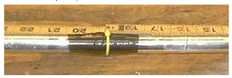
The antenna can be stuck down the back of the shirt, carried, or easily mounted on bicycles, etc. With a little more weatherproofing, it will make a fine dual-band base station antenna of moderate gain (2.2 dbi) and stealthy appearance (paint it the same color as your roof then clamp it to a vent pipe).
